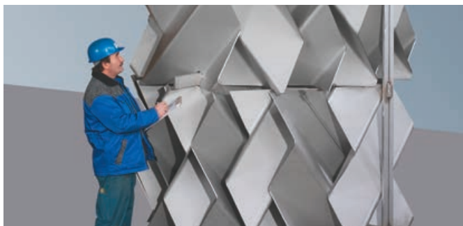
SMV mixer applied for mixing of ethyl benzene and steam in a styrene production plant
