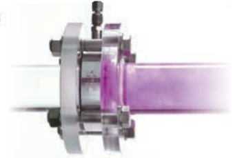
Figure 1. CompaX static mixer with purple additives. Complete mixing at about 3D downstream of static mixer.
