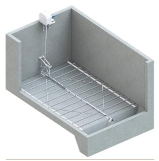
The Zickert bottom sludge scraper uses a reciprocating framework of hydrodynamically shaped profiles mounted on the base of a sedimentation tank.
