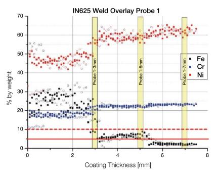
WDX scan results for Alloy 625 overlay probe (3 x 2.5mm, machined to 7 mm)
