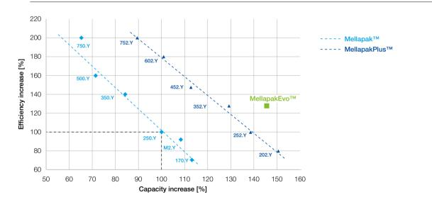
Improvement in capacity and efficiency performance of MellapakEvo, first member of the new product family, tested based on standard organic test mixture under total reflux condition, in combination with advanced MellaTech<sup>™</sup> technology.
