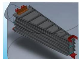
The GIRZ cyclonic inlet device utilizes the momentum of the feed stream inlet in order to generate high g-forces. Defoaming is achieved as gas bubbles are separated from the liquid phase by the centripetal forces in the cyclone tubes. Gas is released from the top of the device and the bottom opening of the cyclones is submerged below the liquid in the separator in order to avoid a gas 'blowout'.
