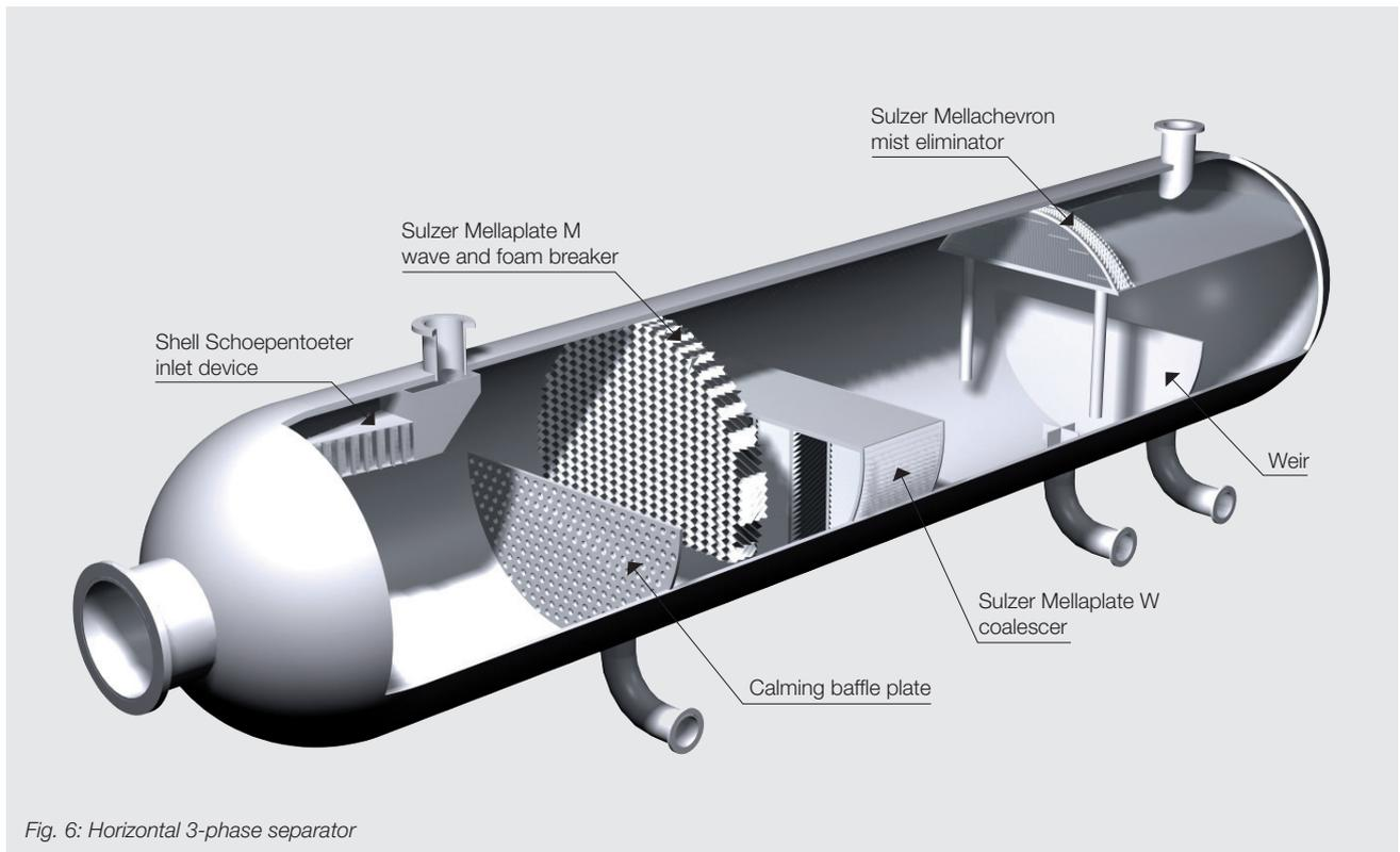
Fig. 6: Horizontal 3-phase separator
