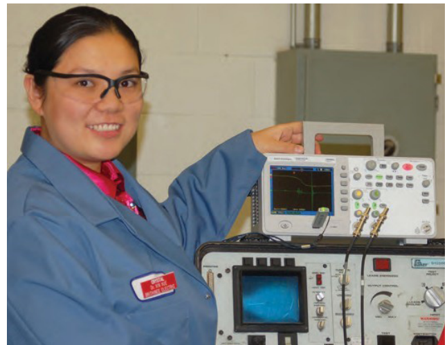
Xin (Crystal) Xue, Ph.D. measures partial discharge inception voltage at Brithinee Electric's Colton plant.
