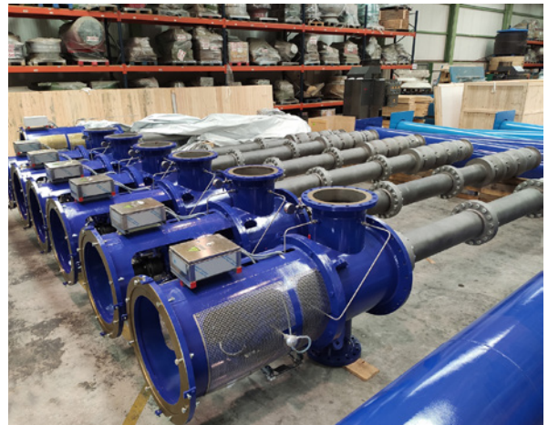
Six 4-stage SJD-CEP condensate extraction pumps were supplied to the power station
