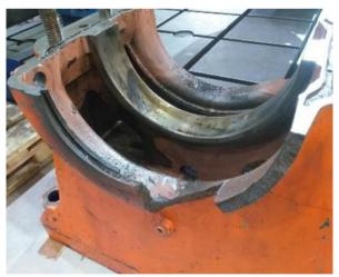
After almost a century of reliable operation, the support bolts installed on one of the turbine shafts at a hydropower plant in West Java finally failed, causing uncontrolled running. This resulted in complete turbine failure and an energy shortage, so the IPP approached several independent service providers (ISPs) for a solution, but no suitable proposal was forthcoming.
