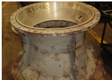
Fabricated stainless steel suction bell
