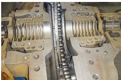
Replace broken blades and balance assembly to ISO G0.665.
