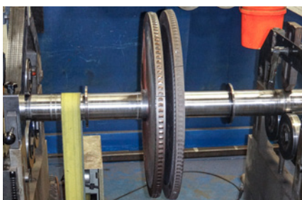
Replace broken blades and balance assembly to ISO G0.665.
