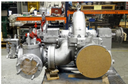
Complete teardown and cleaning. All exposed non-machined areas are painted.
