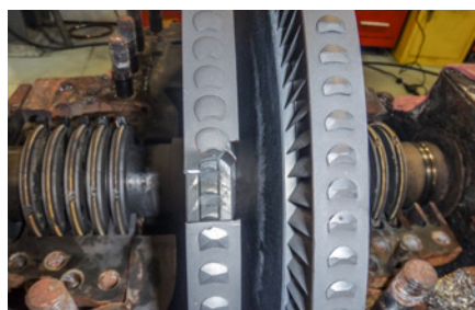
Replace broken blades and balance assembly to ISO G0.665.
