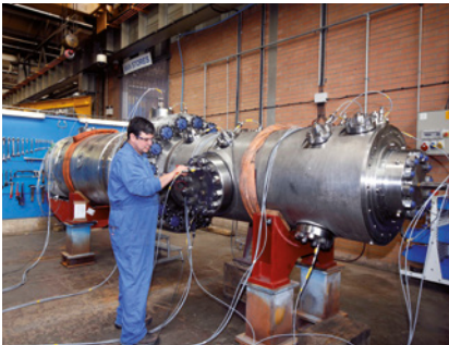
Pump and motor casings being pressure tested.
