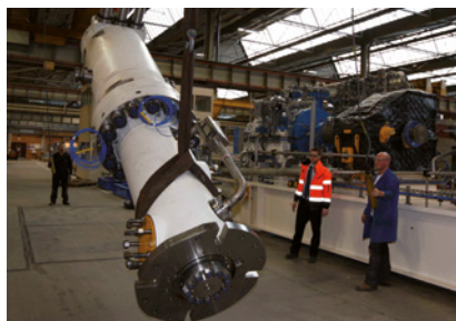
Prototype pump and motor before attachment of cooling coils.
