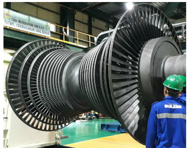
The turbine rotor was also balanced before being reassembled
