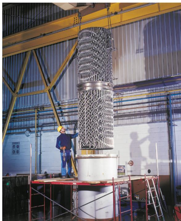
SMR mixer-reactor for heat exchange in exothermic reactions for the chemical/petrochemical industry
