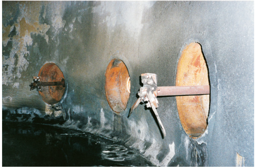
Fig. 2. Agitator with too short a shaft has lost one propeller blade. The farthest agitator has lost all three blades and the one in the middle is in the workshop. All these agitators had 30 kW motors and 1,000 mm propellers. All of them suffered from frequent fatigue failures.
