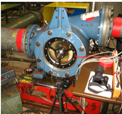
Test on a scale down model of a boiler feed water pump with diffuser
