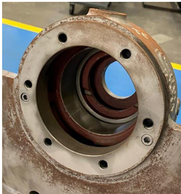
Sleeved housing bore after repair
