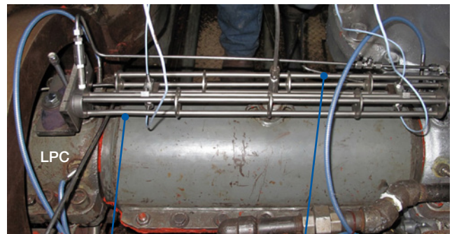
Bar with X-Y proximity probes mounted on LPC bearing housing
