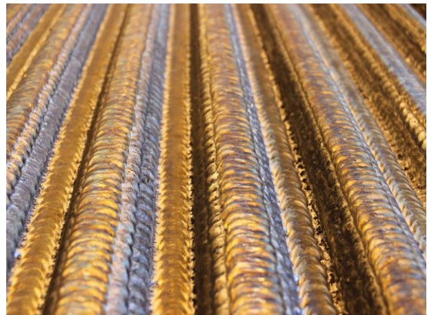
Picture 3: Cladded Panels
