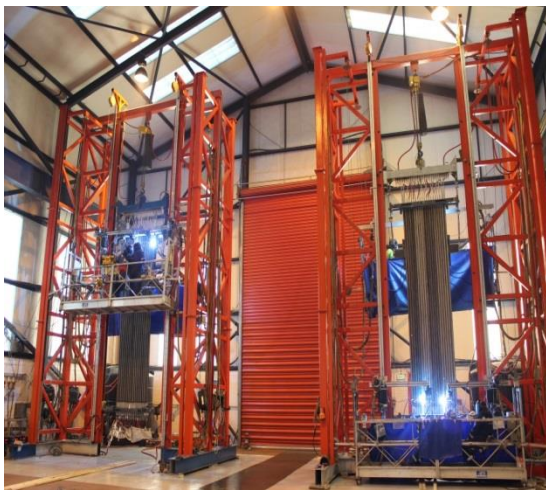
Picture 1: Pulse GMAW membrane wall welding towers.
