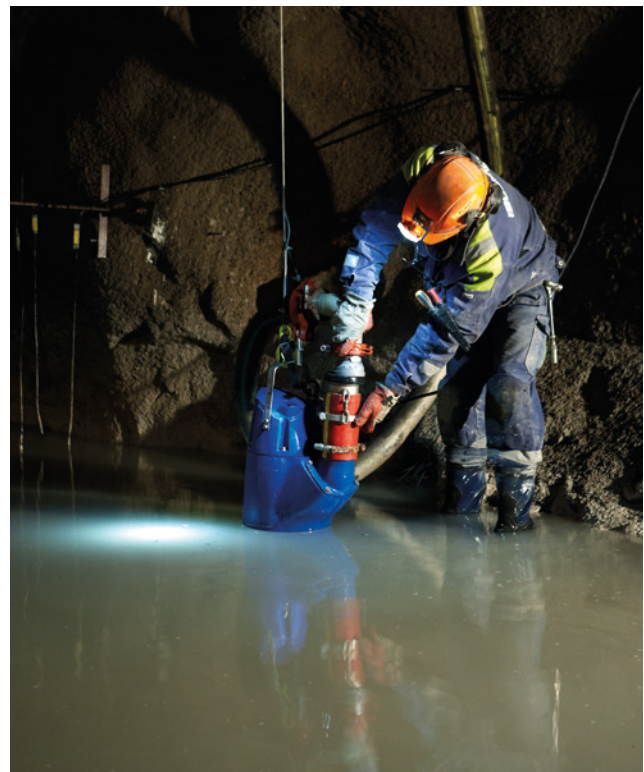
Sulzer's submersible dewatering pumps are excellent for pumping water and dirty water mixed with light abrasives.
