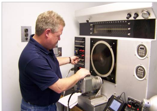
Ignition System Test Stand with Pressurized Spark Rack
