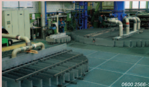
Liquid distributor test to confirm the correct operation range of each distributor
