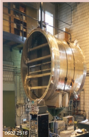
Vibration test, to simulate transportation of assembled columns / cold boxes
