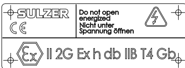
Figure 5b Nameplate ATEX
