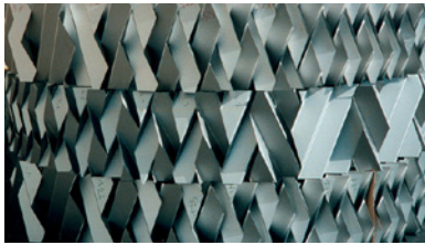
SMV packing for the catalyst stripper
