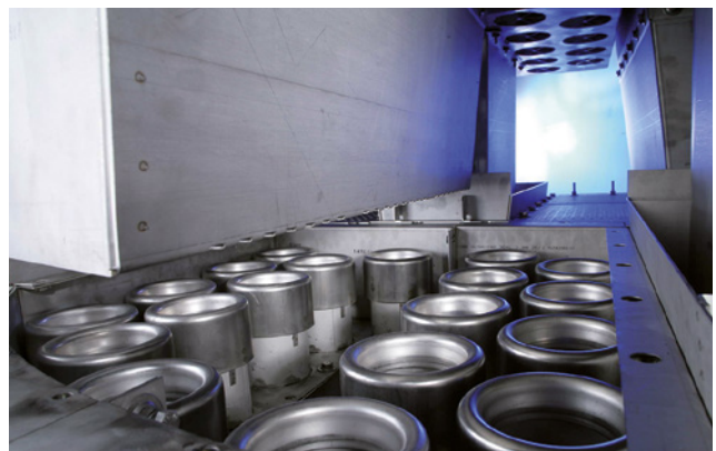
Shell ConSep tray: the ultra system limit high-capacity tray
