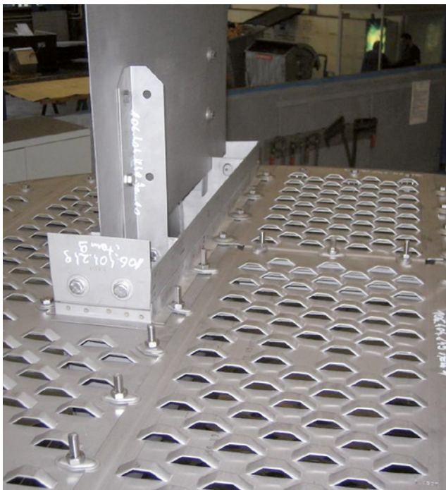
Shell HiFi Plus high-capacity tray equipped with MVG valves
