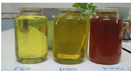
Light Medium Heavy Lube oil samples after revamp
