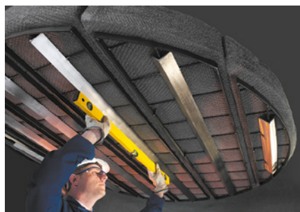
Sulzer Knitmesh™ V-MISTER enhanced performance mist eliminator
