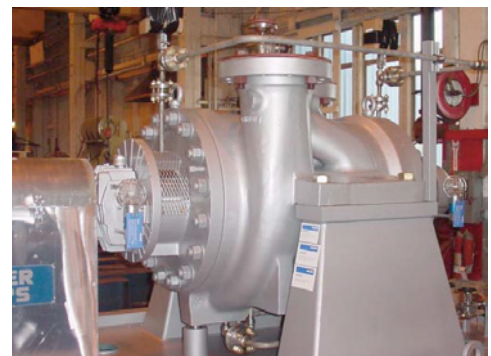
BBS: Single Stage Between Bearing, typically used at high temperature, high flow and high head, that is typically found in residue and the bottom Pump Around of main fractionators
