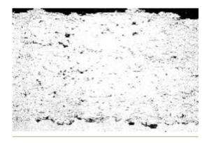
250X cross-sectional photomicrograph of a typical HICoat H64 coating. Coating thickness typically measures 4-6 mils, but can be applied in excess of 25 mils.
