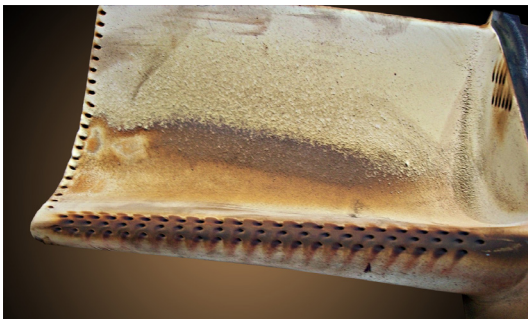
7FA 1st stage bucket after service
