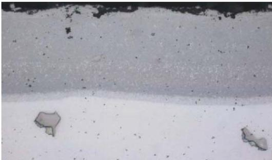
High temperature hot corrosion is of two types: type I and type II. Type I occurs above 1,650°F (900°C) and type II occurs between 1,200°F (650°C) to 1,470°F (800°C). In each of these types of hot corrosion a salt of some kind (e.g. Na<sub>2</sub>SO<sub>4</sub>) must be present, and the rate of metal degradation is much higher than other forms of corrosion.
