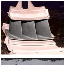
High temperature hot corrosion is of two types: type I and type II. Type I occurs above 1,650°F (900°C) and type II occurs between 1,200°F (650°C) to 1,470°F (800°C). In each of these types of hot corrosion a salt of some kind (e.g. Na2SO4) must be present, and the rate of metal degradation is much higher than other forms of corrosion.
