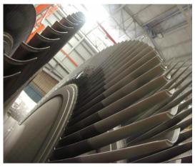
Hardface coatings, particularly HVOF (High Velocity Oxygen Fuel) chrome carbide coatings, have multiple applications in all types of turbomachinery. HVOF chrome carbide coatings are effective in combatting most wear such as solid particle erosion, fretting, abrasion, and cavitation, as well as potentially reducing repair intervals for your coated component.
